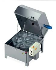
The aqueous Hot Washers use temperature and a pressure chemical action to clean and dry components in an automatic process. This is safe and cost effective.
